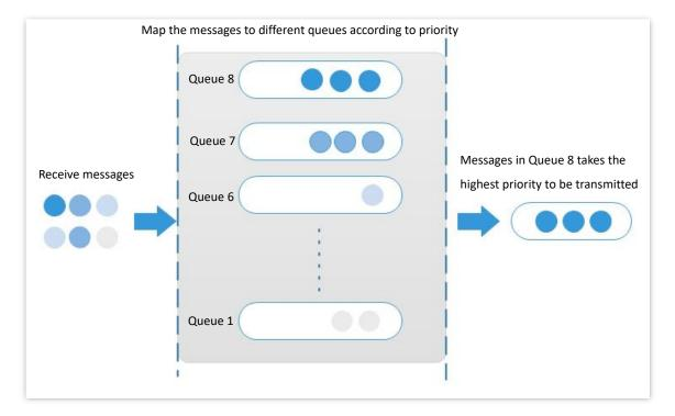
Strict priority scheduling algorithm is specially designed for critical service applications. An important feature of critical services is that they demand preferential service in congestion in order to reduce the response delay.
