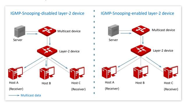
IGMP snooping only forwards data to the specific receivers through the layer-2 multicast, providing the following advantages:
